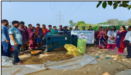
Power operated finger millet thresher for threshing finger millet
